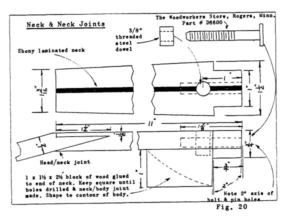
and the neck is shown in Fig. 20. These two pieces are joined and glued in the "square" and then shaped to proper form after the joint is dry. This makes clamping a lot easier. A suggested head shape is shown in Fig. 21. The head drops back 15° from the neck.
